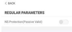
figure 7-16 NS Protection(Passive Valid)
