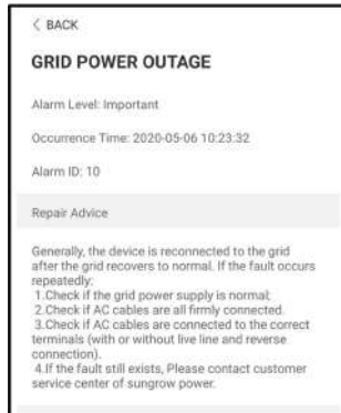
figure 7-9 Detailed Fault Alarm Information
