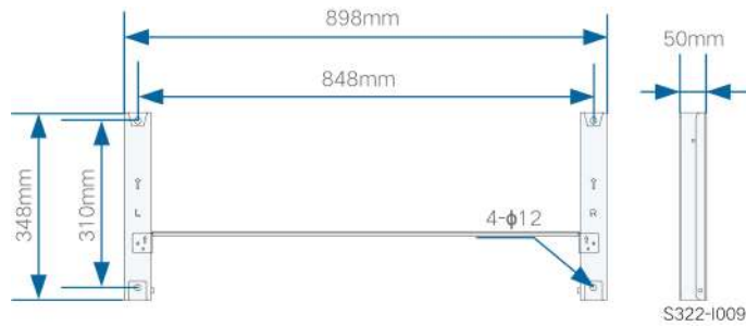
figure 4-1 Dimensions of Mounting-bracket
