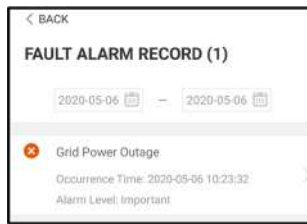
figure 7-7 Fault Alarm Record
