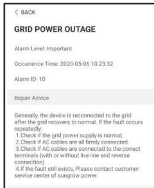
figure 7-8 Detailed Fault Alarm Information
