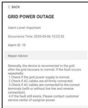
figure 7-9 Detailed Fault Alarm Information
