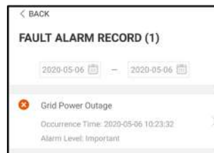
figure 7-8 Fault Alarm Record
