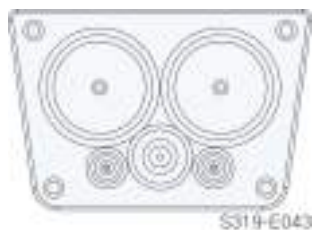
figure 5-4 Sealing Plate for Two Wires per Phase with Multi-core Cable
